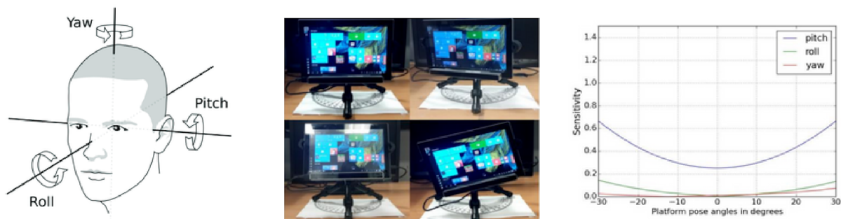
Fig 7.1 (a) Gaze Yaw and Pitch Angular Accuracies (b) Shows the different orientations of the eye tracker in neutral position (top left) and (clockwise from top) roll, pitch and yaw variations. (c) Shows the gaze error sensitivity to orientations of the tablet when eye tracking is performed on it.
